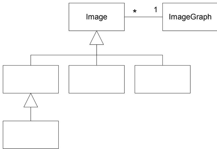
A class diagram introducing the Image and ImageGraph types showing that the Image type is the root type for all value object types and sub-types, or more importantly, the Image type structure mirrors the Imageable type structure. The ImageGraph class manages the namespace for a give Image graph.
