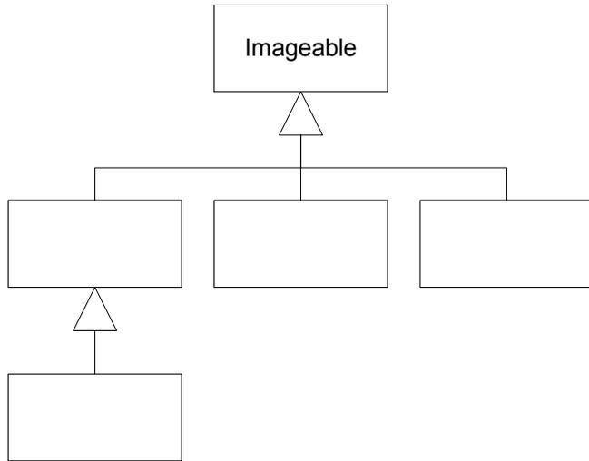
A class diagram introducing the Imageable type (or possibly interface) showing that it is the root type for all business object types and sub-types.
