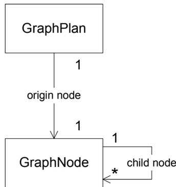
A class diagram introducing the GraphNode class GraphPlan classes. The GraphPlan is purely optional, it would allow trees of GraphNode instances to be named (versioned), persisted, and shared across components of the architecture and between threads concurrently.
