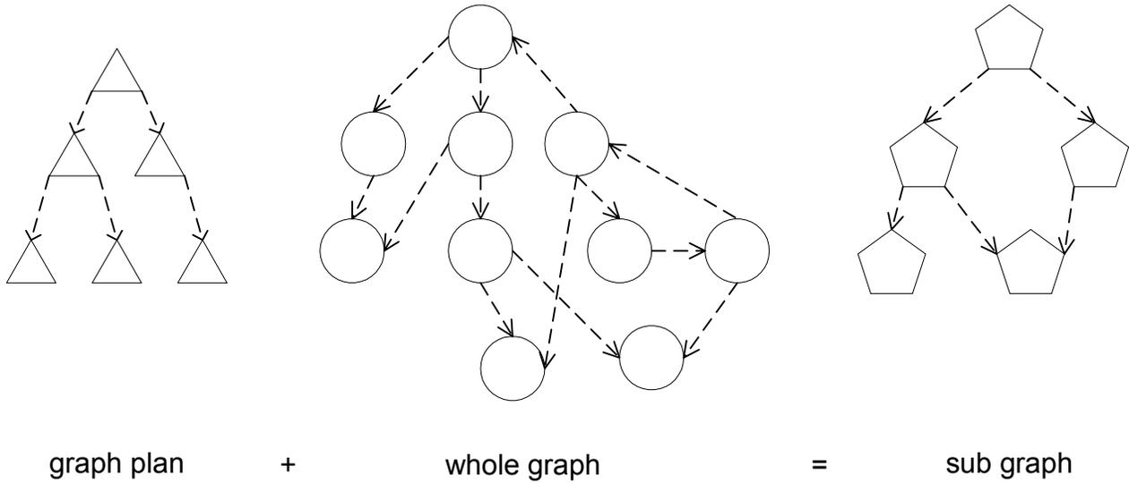
A conceptual diagram showing how graph plans are simply trees used to describe portions of whole graphs.
