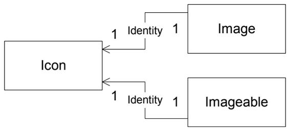
A class diagram introducing the Icon class and its relationship with the Image and Imageable classes. Note that two Imageable and Image instances represent the same entity if they have equivalent Icon instances.
